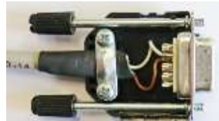
Figure 4; CAN cable SE device ↔ SIOS gateway
