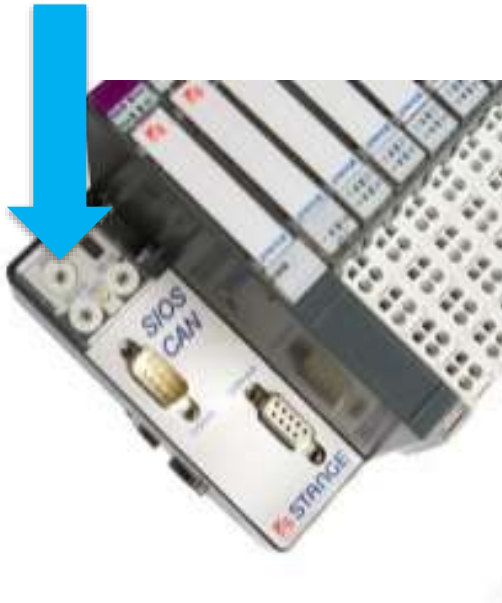
Figure 2; Baud rate rotary switch
