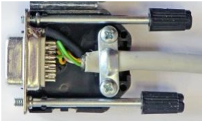
Figure 4; CAN cable SE device -<=> SIOS gateway
